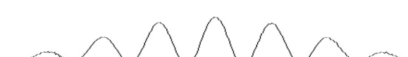
Fig. 8. The sum of 240 half-second exposures (120 s accumulation time) with 2 \times 2 binning. The graph and image grayscale is 0–2000 counts.
