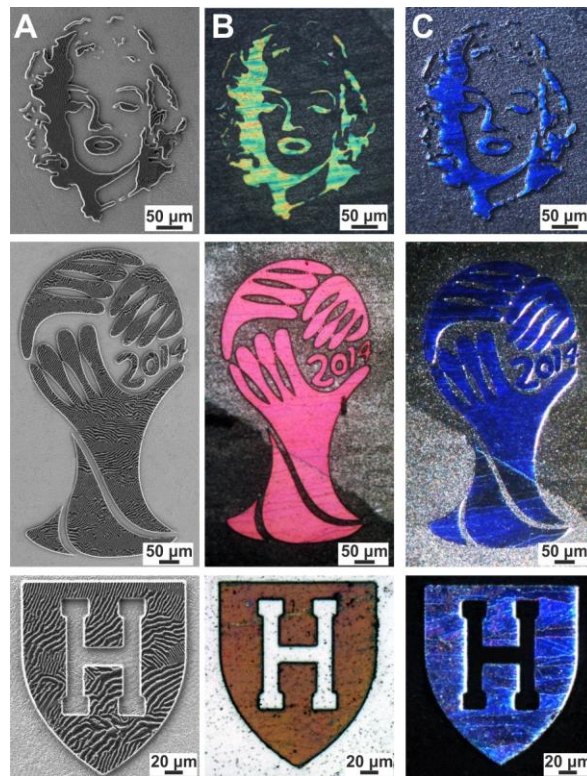
Figure 4. Structural color imaging at micron scale. A) SEM images of hierarchical inverse opal structures; B-C) microscopy images taken with illumination normal (B) and off-normal to the surface (C). The images show real, dynamic structural color that blue-shifts with increasing illumination angle.
