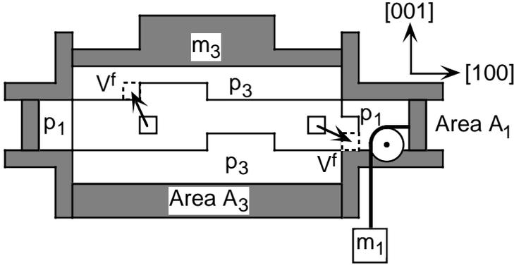
Fig. 2. Work done upon vacancy formation in crystal (middle) with stepped surfaces free of extended defects. Pressures,  $p_1$  and  $p_3$ , of incompressible fluids in contact with (100) and (001) faces, respectively, maintained by pistons driven by masses  $m_1$  and  $m_3$ . Crystal volume changes by  $V^f$  upon vacancy formation at (100) or (001) surface, but work done against gravity differs.
