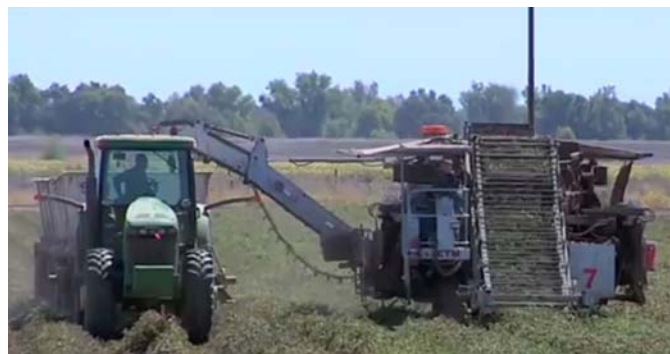
Figure 2: Image of tomato harvester (right) and trailer (left)
