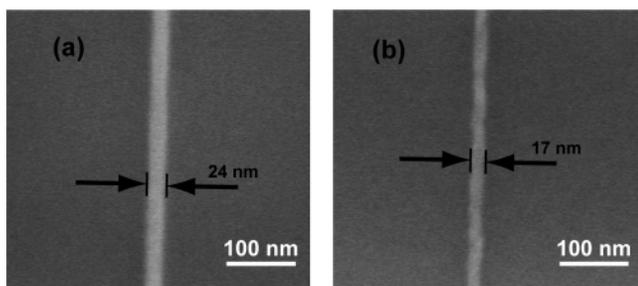
**Figure 3.** SEM analysis of sub-30 nm wide Cr lines on a bulk silicon substrate. Both structures were defined on 20 nm ice resist layers and subsequently metallized with 8 nm Cr. (a) 30 keV line, 4.5  $\mu\text{C}/\text{cm}$  dose. (b) 20 keV line, 4.4  $\mu\text{C}/\text{cm}$  dose.
