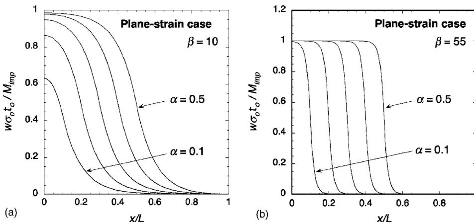
FIG. 7. Normalized membrane deflection as a result of ion implantation for the plane-strain case: (a) membrane with a small value of  $\beta$ ; (b) membrane with a large  $\beta$  value. Deflections are shown for  $\alpha$  increments of 0.1.
