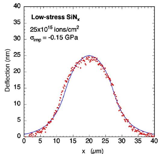
FIG. 9. (Color online) Experimental deflection of a low-stress silicon nitride membrane for the case where a circular region with a 15  $\mu\text{m}$  diameter was implanted with  $25 \times 10^{15}$  Ga<sup>+</sup> ions/cm<sup>2</sup>. The solid line is the shape predicted by the model.
