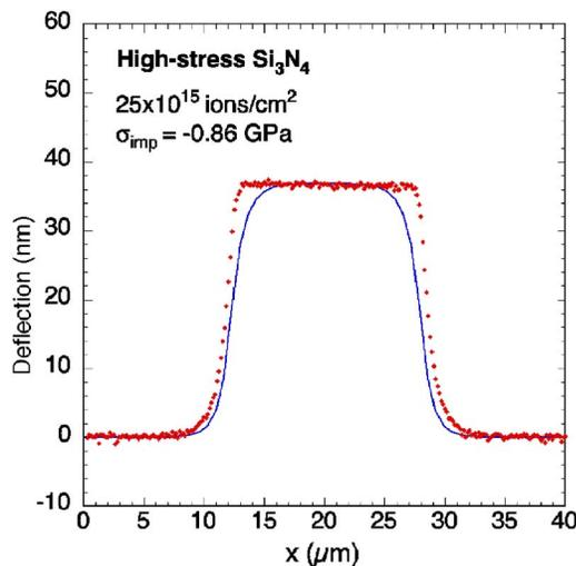
FIG. 10. (Color online) Experimental deflection of a high-stress silicon nitride membrane for the case where a circular region with a 15 μm diameter was implanted with  $25 \times 10^{15}$  Ga<sup>+</sup> ions/cm<sup>2</sup>. The solid line is the shape predicted by the model.
