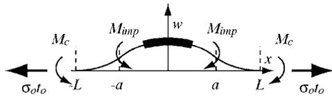
FIG. 6. Schematic illustration of the bending moments exerted on a section of the membrane. Note that the sign of the moments is defined conventionally as shown in the figure.
