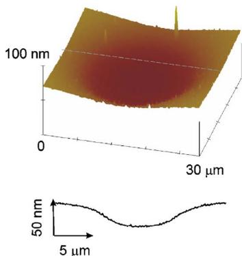
FIG. 4. (Color online) AFM image showing the depression induced in a freestanding low-stress silicon nitride membrane by ion beam irradiation ( $625 \times 10^{15}$  ions/cm<sup>2</sup>) over a circular region. The AFM scan was made on the back side of the membrane. The AFM sectional profile, shown below the AFM image, reveals the gradual deflection of the membrane.
