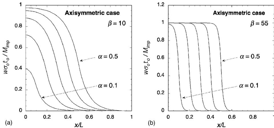
FIG. 8. Normalized deflection as a result of ion implantation in a circular region for an axisymmetric membrane with a small  $\beta$  value (a) and a large  $\beta$  value (b). Deflections are shown for  $\alpha$  increments of 0.1.
