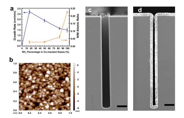
**Figure 2.** (a) Growth rate and N/Ni atomic ratio plotted versus the  $NH_3$  percentage out of the  $NH_3/H_2$  co-reactant mixture (60 sccm in total) used during DLE-CVD process; (b) Taping-mode AFM image on the surface of Ni film. (c) Cross-section SEM images of a silicon trench test structure; (d) The same silicon trench after Ni deposition, demonstrating the conformality of the deposited film.
