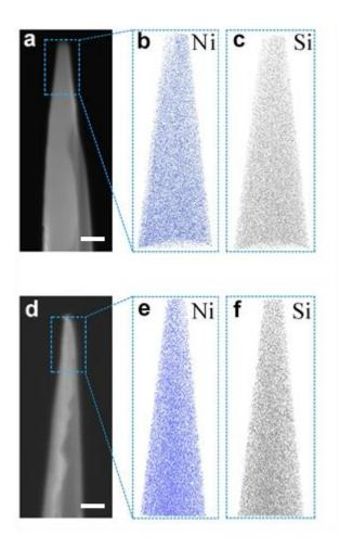
**Figure 4.** Ni and Si elemental atom probe reconstruction images of the specimens from outside (b-c) and deep inside (e-f) of a trench, corresponding with the SEM images shown in (a) and (b), respectively. Scale bars denote 100 nm.
