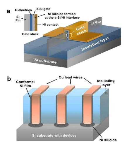
**Figure 1.** (a) Schematic illustration of Ni silicide applied on Fin-FET, improving the contact between a-Si gates and lead wires; (b) Formation of Ni silicide deep inside hole structures facilitates the contact between copper TSVs and silicon substrates with devices.
