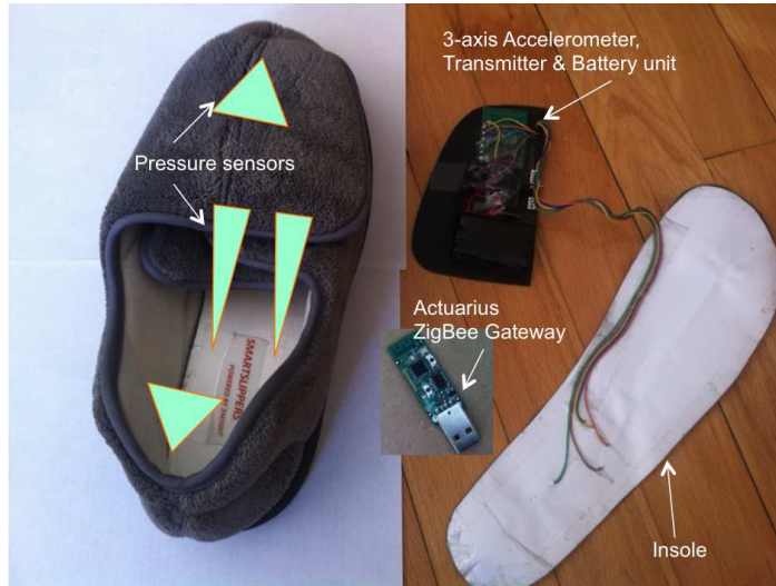
Figure 6.1: SmartSlipper™: Shoes, insoles and associated hardware. (Left) The shoe and location of four pressure sensors on the shoe. (Right) The insole containing the pressure sensors and a powered unit that goes in the inside strap of the shoe. The powered unit contains the ZigBee wireless transmitter as well as the acceleration sensors. (Center) USB dongle that acts as the gateway for ZigBee data on the receiving end.
