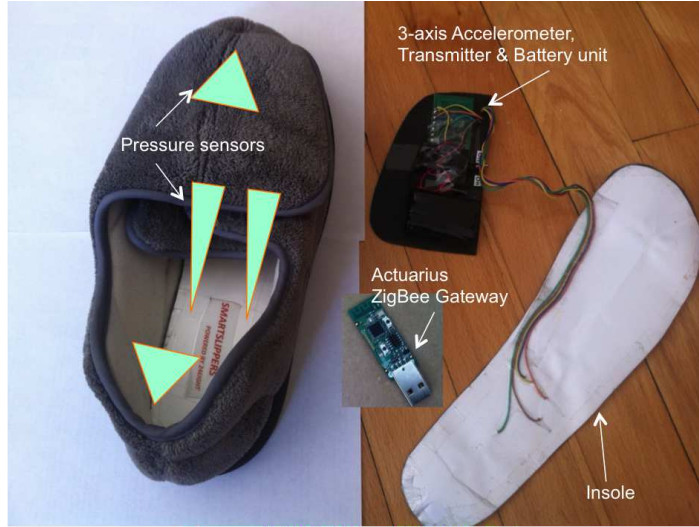
Figure 6.1: SmartSlipper TM : Shoes, insoles and associated hardware. (Left) The shoe and location of four pressure sensors on the shoe. (Right) The insole containing the pressure sensors and a powered unit that goes in the inside strap of the shoe. The powered unit contains the ZigBee wireless transmitter as well as the acceleromotion sensors. (Center) USB dongle that acts as the gateway for ZigBee data on the receiving end.
