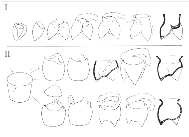
Figure 6-2 - The stages of manufacture of fendang (I) and Liedangli (II) after Kaogu (2006: 42)
