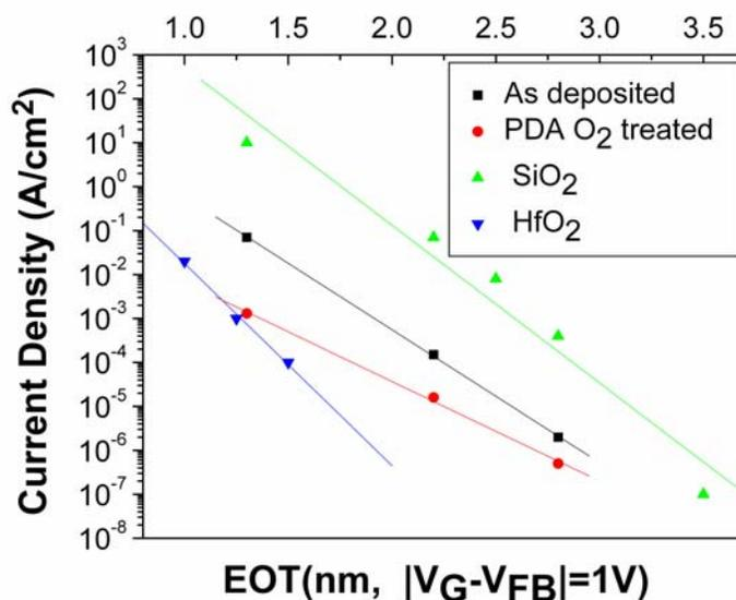
Figure 6. Leakage current density at 1 V of  $|V_G - V_{FB}|$  with respect to EOT for  $\text{LaAlO}_3$  (both as-deposited and samples treated with  $\text{O}_2$  after deposition),  $\text{SiO}_2$ , and  $\text{HfO}_2$ .
