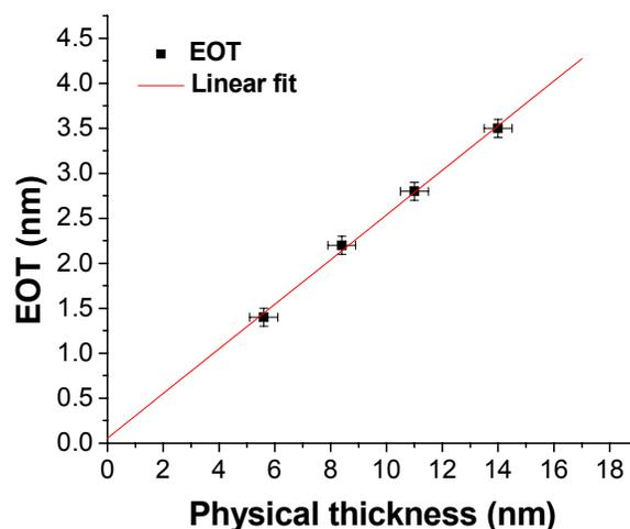
Figure 4. EOT plotted as a function of physical thicknesses of LaAlO<sub>3</sub>. The intercept from the linear fit is  $0.05 \pm 0.09 \text{ nm}$  and the dielectric constant is  $15 \pm 1$ .
