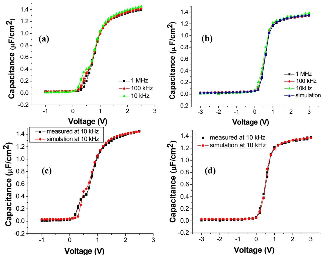
Figure 1. Comparison of  $C$ - $V$  curves at different frequencies between (a) the as-deposited sample and (b) PDA  $\text{O}_2$  treated sample. A simulation curve is at 1 MHz is shown in (b); (c) as-deposited and simulated at 10 kHz; (d) PDA  $\text{O}_2$  treated sample and simulated at 10 kHz.
