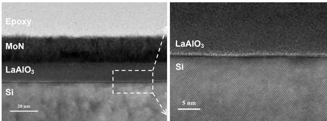
Figure 3. High resolution TEM micrographs of a MoN/LaAlO<sub>3</sub> stack on Si. After deposition, the LaAlO<sub>3</sub>/Si was treated in  $O_2$  at 300 °C for 10 min, and then the whole stack underwent RTA at 400 °C for 4 min in forming gas prior to imaging. Both MoN/LaAlO<sub>3</sub> and LaAlO<sub>3</sub>/Si interfaces are sharp and smooth.
