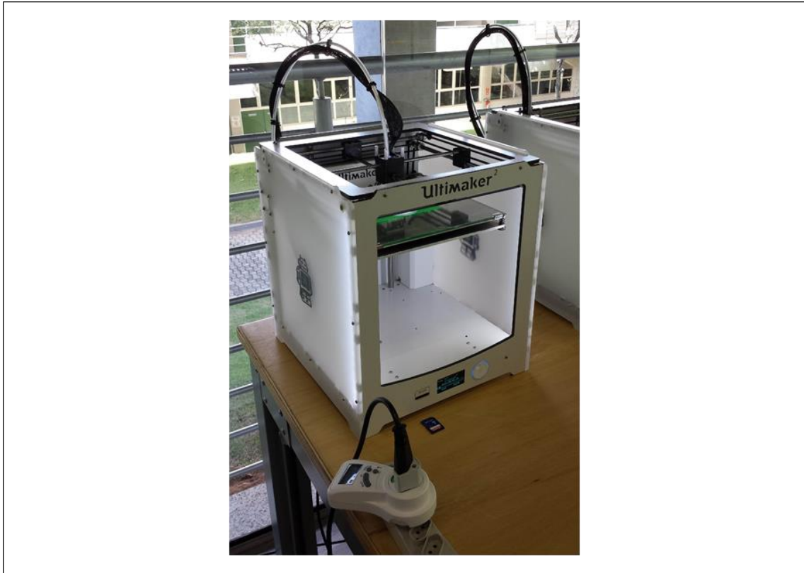
Figure 7. Desktop 3D printer and watt-meter plugged into a powerline.
