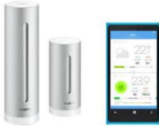
Figure 20. Netatmo devices used to measure the indoor environment. A screenshot of the results captured from the device.
