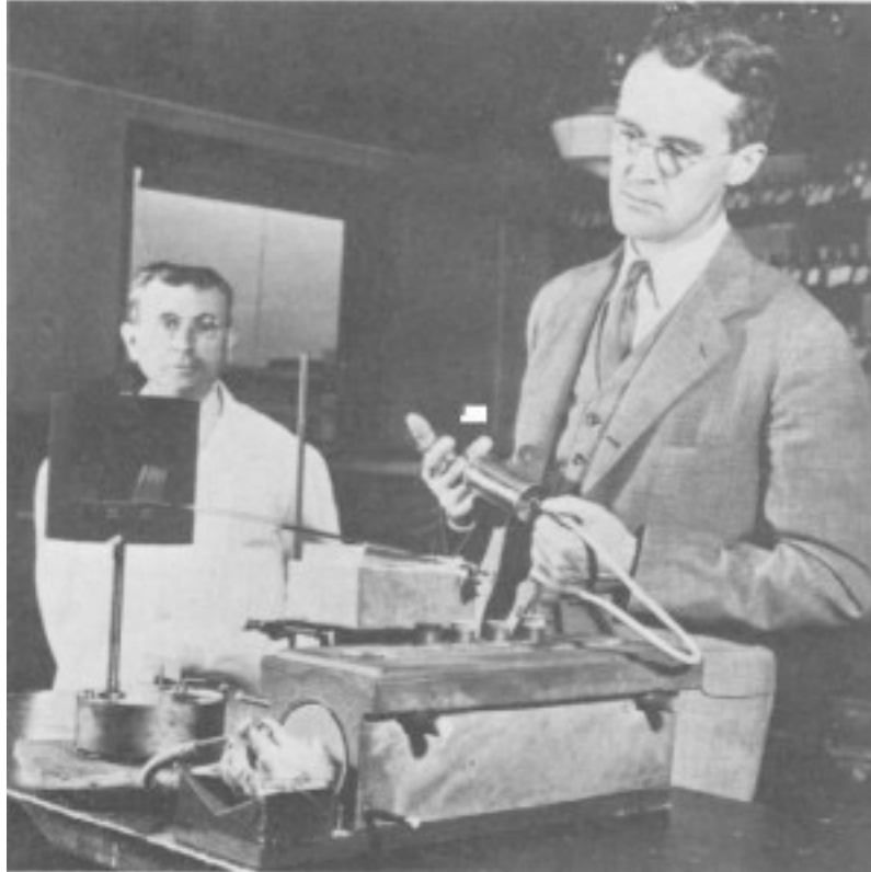
Figure 13. Phillip Drinker applies negative and positive pressure to ventilate a curarized cat while assistant Louis Freni looks on. Source: Catherine Drinker Bowen, Family Portrait (Boston: Little, Brown, 1970), 239.
