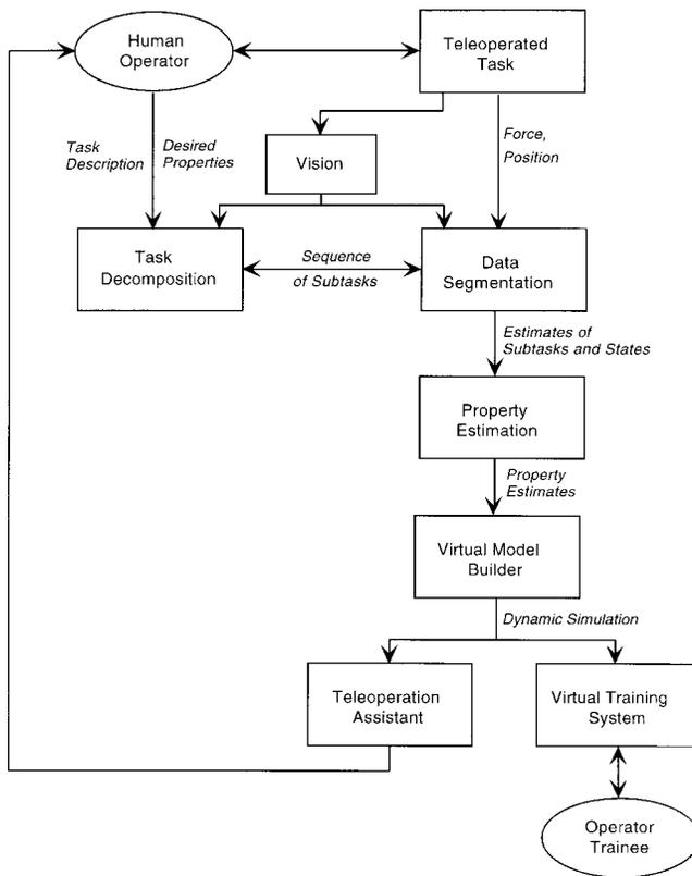
Figure 2. Flow diagram of the environment identification problem.
