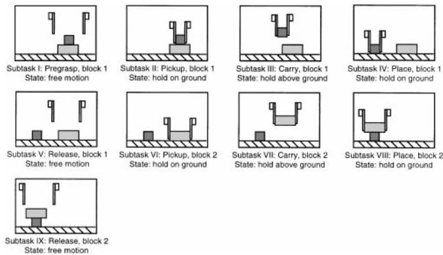
Figure 3. Block-stacking task.
