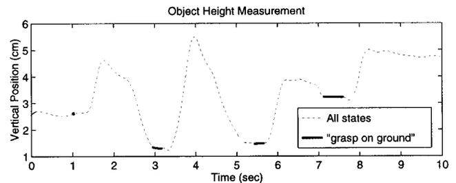
**Figure 9.** Object heights. The solid portions are the segments of data used for height estimation. Object 2 height is the difference between the first and second solid lines, while object 1 height is the difference between the third and fourth solid lines.
