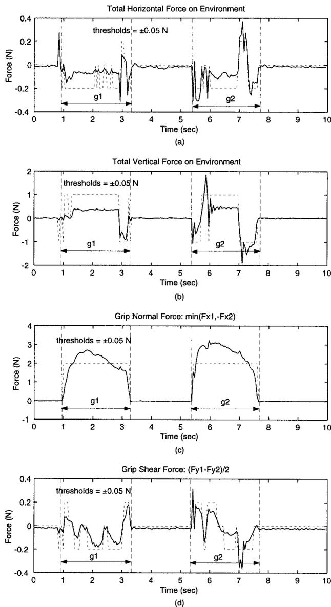
**Figure 6.** Forces: (a) Total horizontal force on environment; (b) Total vertical force on environment; (c) Grip force; (d) Vertical shear force. Legend:  $g1$  = grasping object 1;  $g2$  = grasping object 2.
