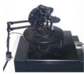
(c): PHANToM™ device used as robotic probe.
