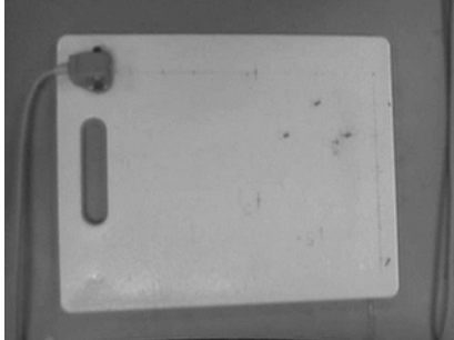
(b): Calibration fixture with tracking receiver and calibration pins attached.
