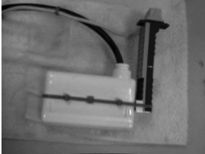
(a): Ultrasound probe with offset tracking receiver attached.
