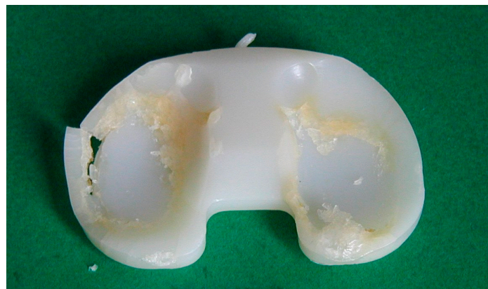
Figure 3. Retrieved polyethylene tibial insert showing severe wear damage, including severe delamination and wear (10 years in vivo ).
