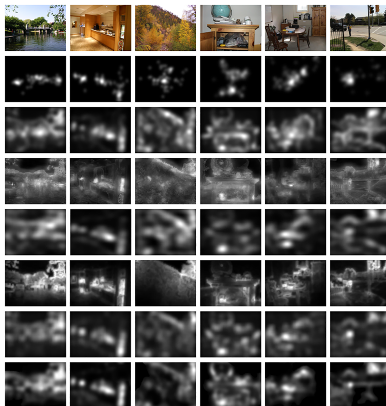
Fig 4. Some sample images and corresponding saliency maps produced by compared models. The first row is original images, and the second row is the human eye density maps. The third to last row are the saliency maps, which are produced by the model of Harel [9], Judd [11], HFT [10], Erdem [12], Lu [13], and our proposed, respectively. The left three images belong to the MIT database, and the right three images belong to the Toronto database.
