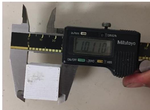
Figure 21. Testing of Phase 1 test print dimensions and tolerances.
