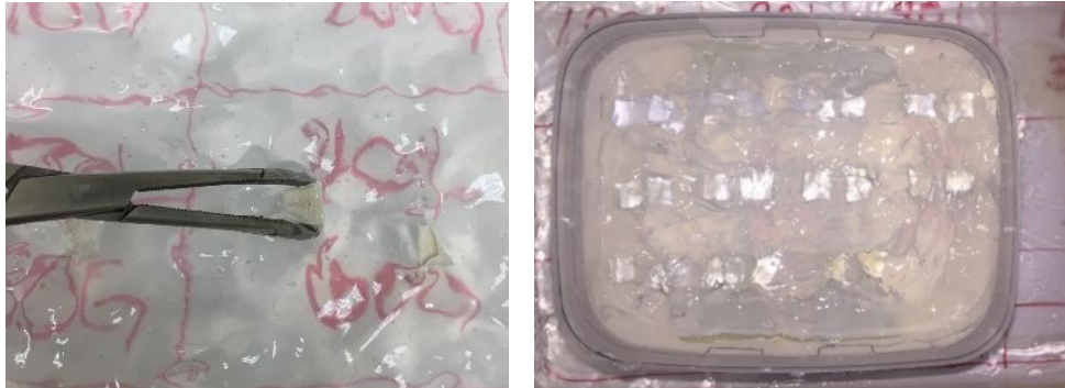
Figure 48. Forceps were used to place blocks within the gel (left). The completed phantom prototype (right) consisted of three rows of cubes. The first and second rows each had four pairs of blocks, while the third row had three pairs of blocks, for a total of 22 blocks. Blocks are arranged in decreasing Lay-felt proportion from left to right within each row, with the top row containing the highest Lay-felt proportions and the bottom row containing the lowest Lay-felt proportions.
