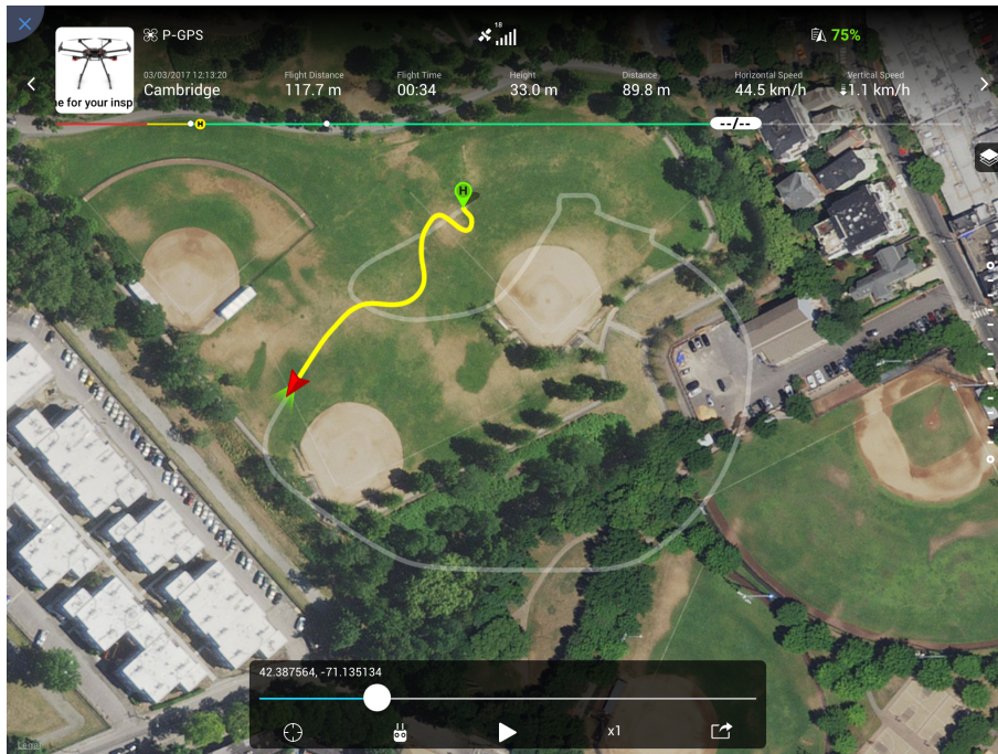
Fig. 5.5 Screenshot of sample test flight trajectory at Danehy Park, Cambridge MA from DJI Go application. This particular test flight lasted 2:29 min, covering 656.7 m and reaching a maximum altitude of 38.0 m.
