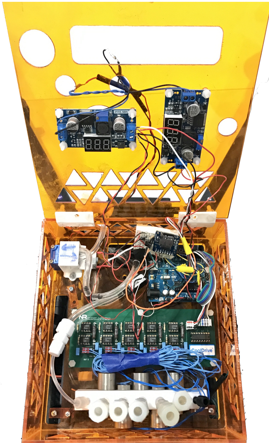
Fig. 4.2 Fully assembled sampler instrument. The instrument enclosure is assembled out of acrylic with holes to reduce drag and mass. Individual components are mounted directly to the bottom panel of the enclosure and the top panel is designed to open for access to internal components.
