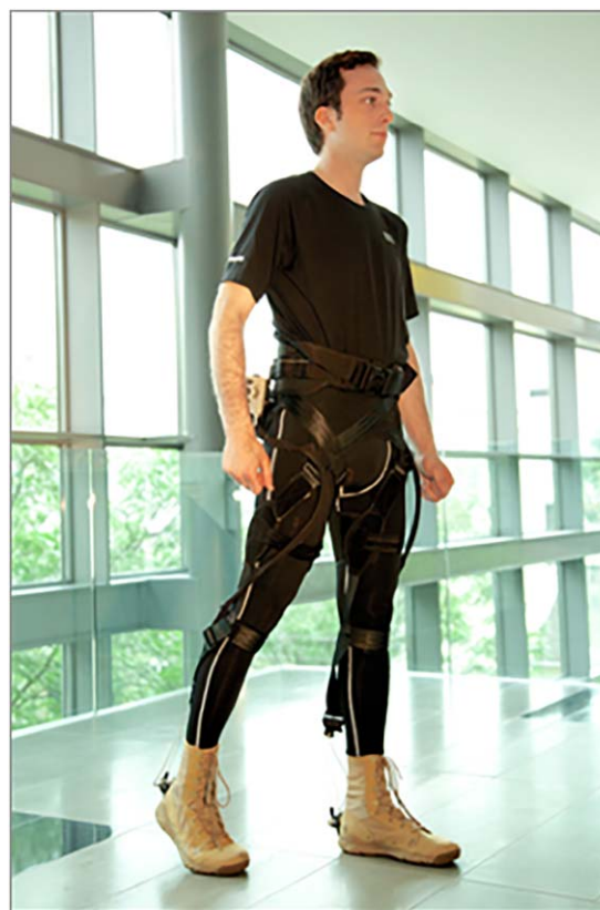
FIGURE 2 Soft exosuits for gait enhancement. Lightweight and flexible exosuits made of fabrics with integrated artificial muscles and robotic control offer a new way to assist children and adults with movement disorders such as stroke, multiple sclerosis, and Parkinson’s disease, the elderly in maintaining or restoring gait or soldiers, firefighters, paramedics, and others whose jobs require them to carry extremely heavy loads. [Work from Conor Walsh and the Wyss Bioinspired Robotics Platform] 8
