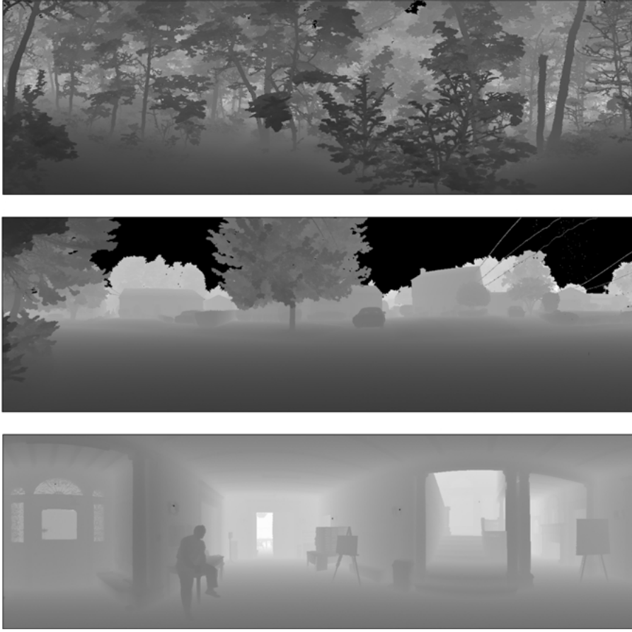
Figure 4. Samples from the Brown range image database by Huang and Lee. The gray values code for log-range values.
