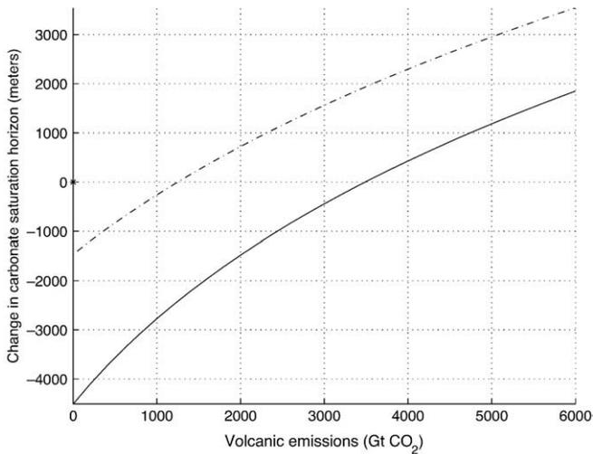
**Fig. 7.** Modeled change in the carbonate saturation horizon between the last glacial and present interglacial for various volcanic inputs of CO<sub>2</sub> into the ocean–atmosphere system. One scenario considers only changes in CO<sub>2</sub> and temperature (dashed line), and the other also includes organic storage of carbon on the continents (solid line). Our estimate of ~3000 Gt of volcanic CO<sub>2</sub> emissions requires little change in the carbonate saturation horizon.
