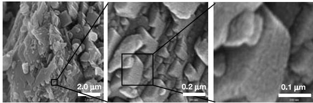
**Figure 4** Scanning electron microscope images of untreated gouge from San Andreas gouge, with an order-of-magnitude resolution increase from left to right. The gouge samples were mounted onto colloidal graphite coating covering upper portions of platinum trays, and sputter-coated with gold–palladium under vacuum. Note the particles of 0.02–0.05 μm in the middle and right frames.
