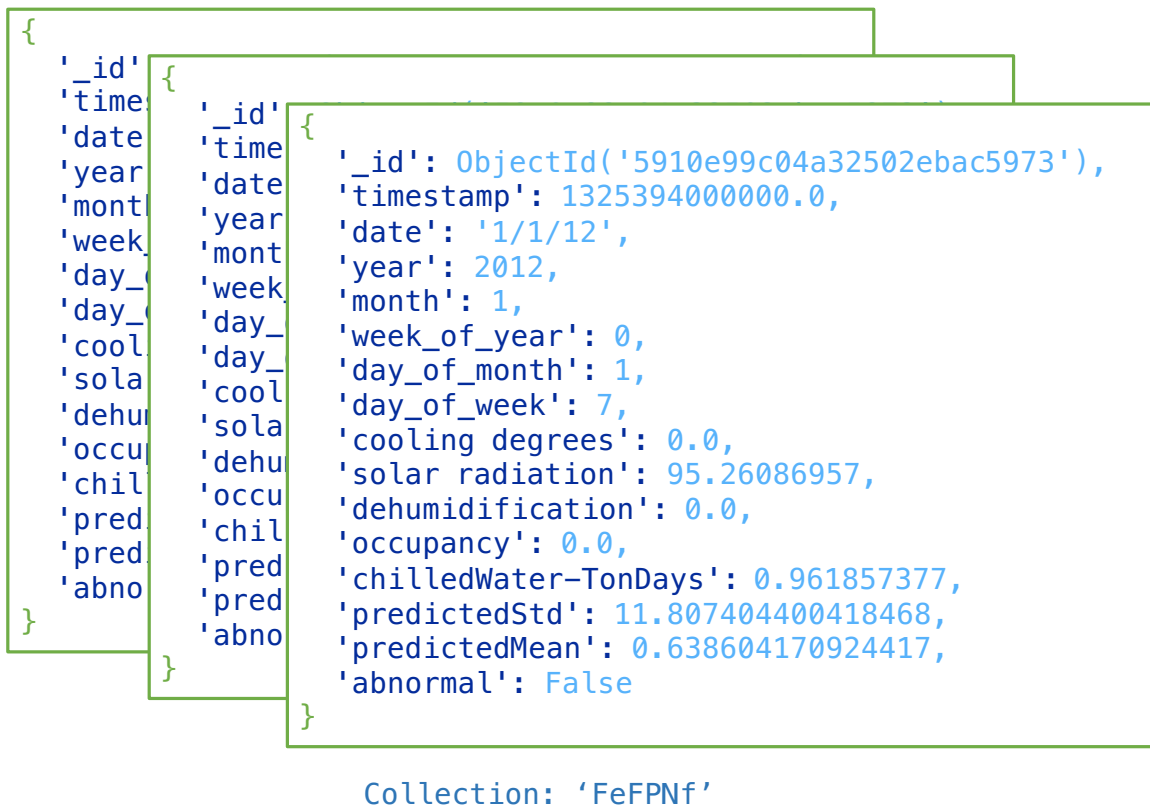
Figure 13 Structure of a collection that stores data uploaded by a user and corresponding processed data
