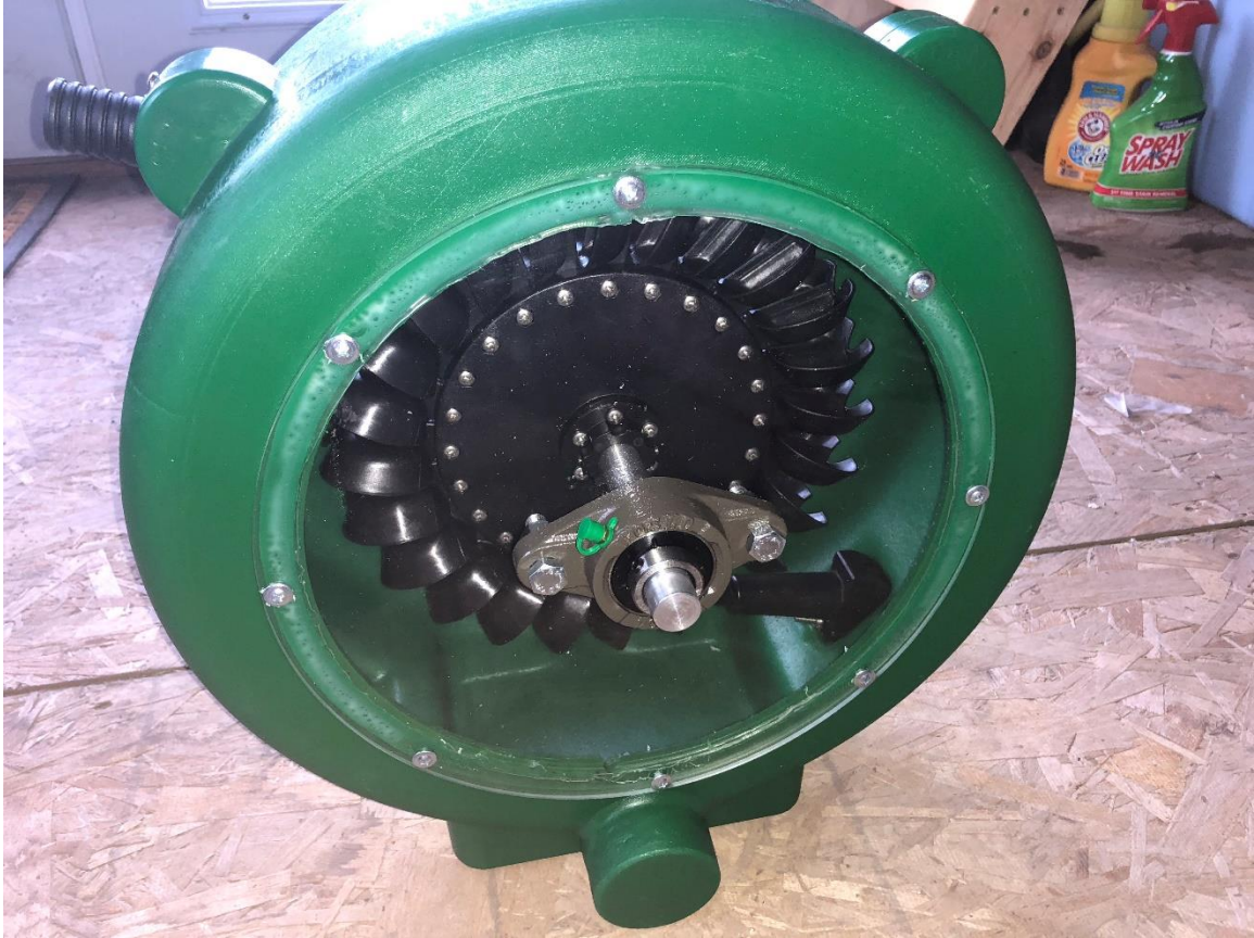
Figure 3. Pelton wheel encased in housing to trap water and gravity feed lower storage tank (photo by author, 2018).
