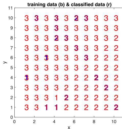
Figure 8.11: A classification neural network with too few nodes calculates labels (red) that cannot match all training data (blue).
