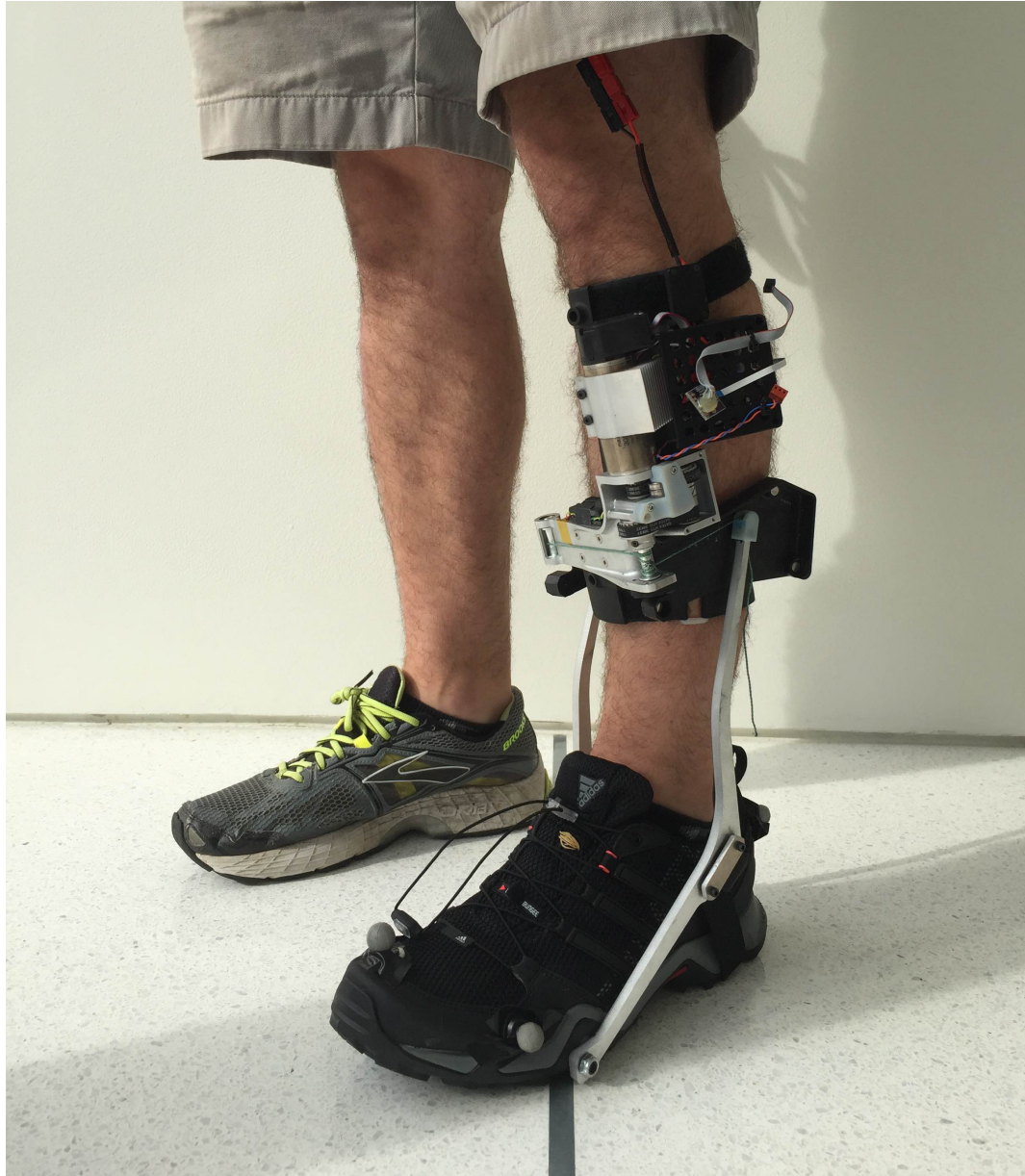
Figure 2: A later iteration of the MIT Media Lab portable autonomous powered ankle exoskeleton featuring low-profile metal struts not utilized in this study. However, the presently described exoskeleton system does feature athletic shoes rather than military boots.
