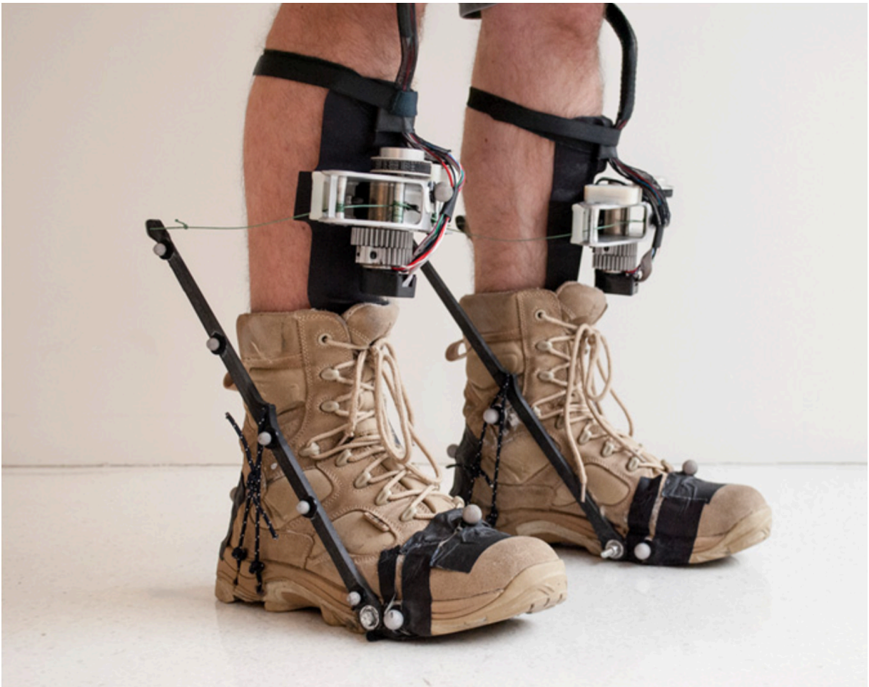
Figure 1: The original Mooney et al. portable autonomous powered ankle exoskeleton, 2014
