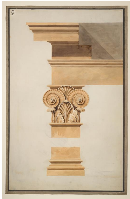
Figure 2.17 Entablature, capital & base for the Ammonite order used by George Dance the Younger at Boydell’s Shakespeare Gallery, a Royal Academy Lecture Drawing commissioned by John Soane.
