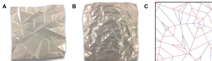
Fig. 1. Examples of crease networks. (A) A 10 cm by 10 cm sheet of Mylar that has undergone a succession of rigid flat folds. (B) A sheet of Mylar that has been crumpled. (C) A simulated rigid flat-folded sheet. The sheet has been folded 13 times. Ridges are colored red, and valleys are blue.
