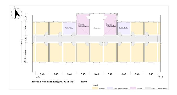
Figure 4-76 Redrawn second plan of building No. 30
