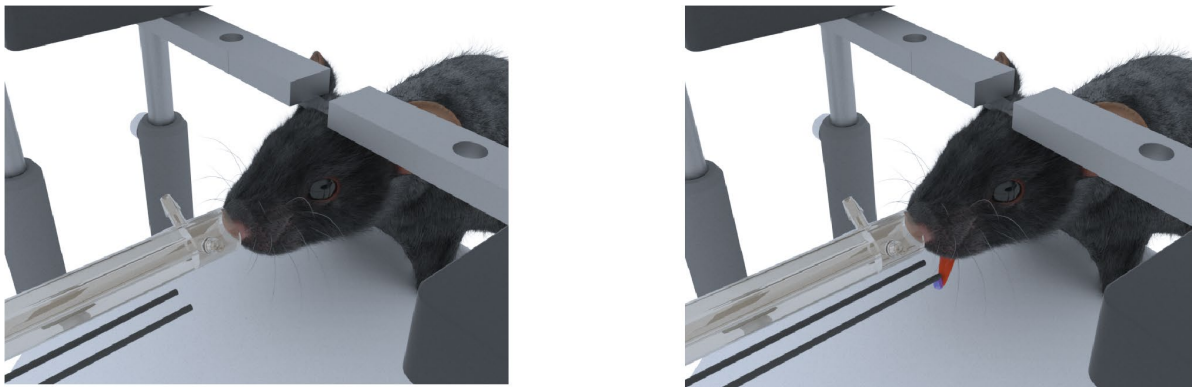
Figure 5.5. left: Lickport is away from the mouse during wait and sampling period. Right: Lockport is reachable by the mouse during the go period.
