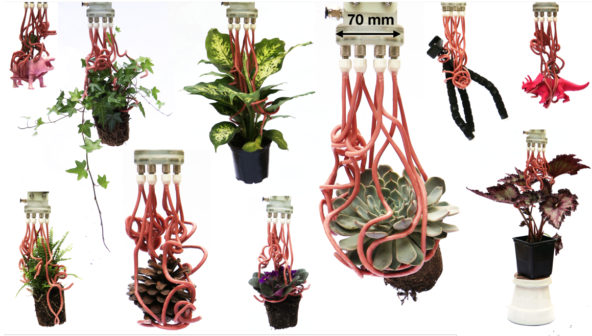
Figure 5.17: Topologically complex household objects held by a 12-filament entanglement gripper.
