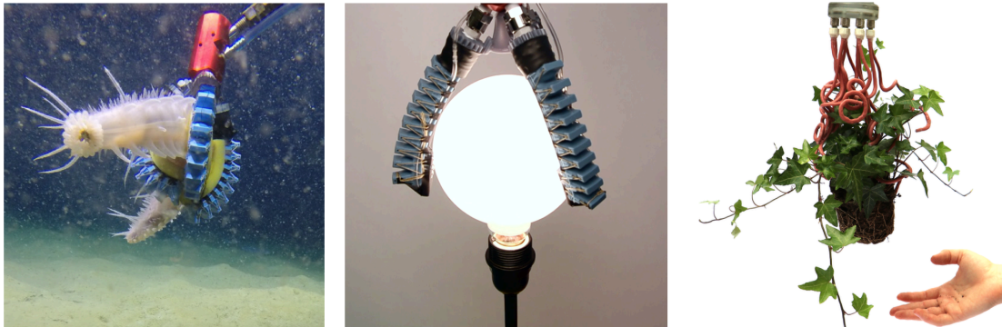
Figure 1.1: Three demonstrations in which the design and fabrication of a soft gripper was used to specifically tune the contact interface to adapt to a target object. (Left) A hydraulically actuated gripper applies a gentle, conformal, and secure grasp to a holothurian, 1800 m under water. (Center) A pneumatically actuated gripper installs a light bulb with the help of controllable friction pads on its finger tips. (Right) An entanglement gripper applies distributed contacts to adapt to and gently lift an ivy plant.
