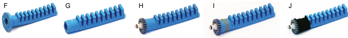
Figure 2.9: Pictures showing the hardware installation for bellows-type actuators. The hardware allows for modular attachment to a deep-sea gripper palms. (F) The soft core is removed from the actuator and (G) the flange is removed. (H) Connective hardware is glued into the base of the actuator, (I) reinforced with Kevlar thread, (J) and covered with heat-shrink tubing. The finished length of the actuator from connector to finger tip is 128 mm.
