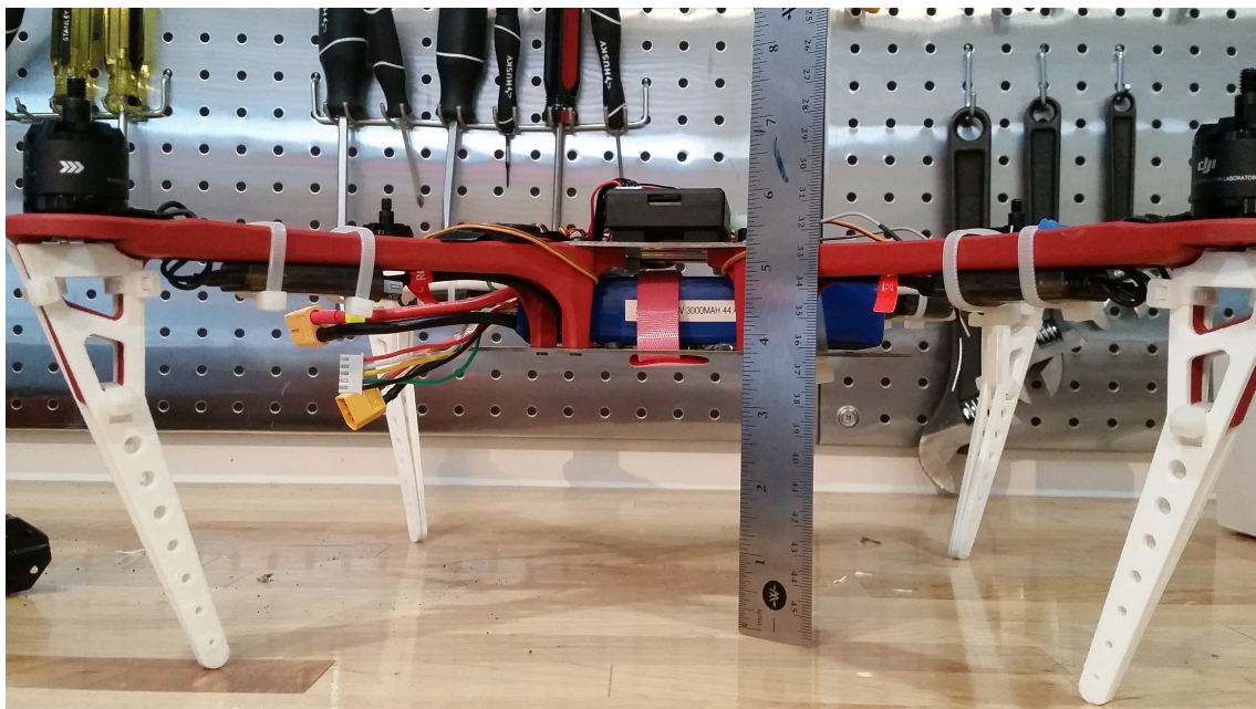
Figure 2-17: The UAV with shorter and more spread out landing gear.
