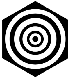
Figure 1-4: The landing marker used in the system developed by Lange et al.
