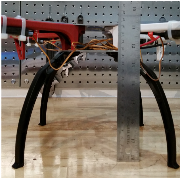
Figure 2-16: The UAV with taller landing gear.
