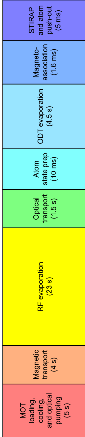
Figure 3.1: Experimental steps in the production of ultracold KRb molecules and their durations.
