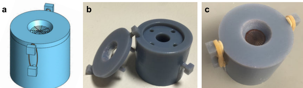
Figure 3.4. Custom-built holders for digital opto-electronic holography (DOEH) and laser Doppler vibrometry (LDV). (a) Customized 3D printed holder is designed for use in DPOE and LDV experiments. (b) 3D printed holder open, without a graft. (c) 3D printed holder containing a graft clamped and held together by rubber bands.
