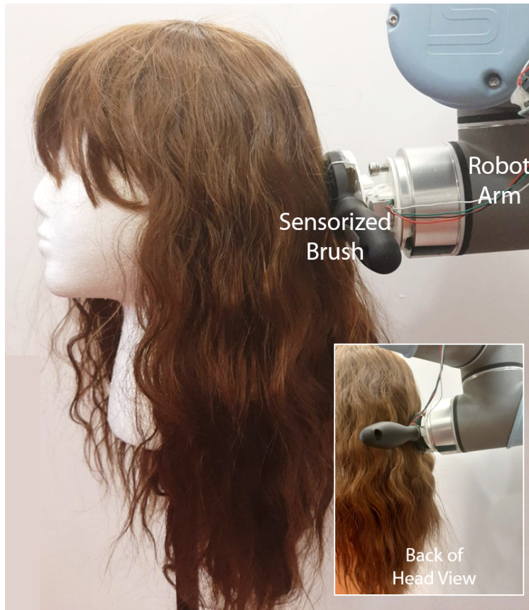
Figure 3.1: Experimental setup for the investigation of robotic hair brushing showing the wig, sensorized brush and robot arm.
