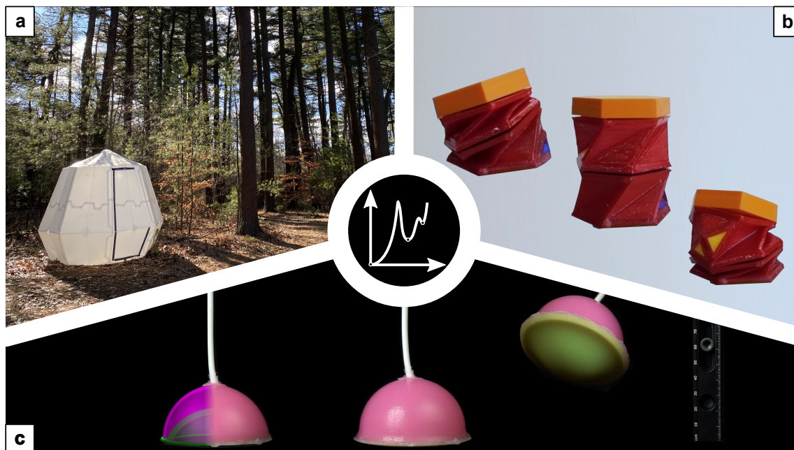
Figure 5.1: Contributions. (a) Meter-scale inflatable and multistable structures (b) Multimodal soft actuators. (c) Fast soft robotic jumper.
