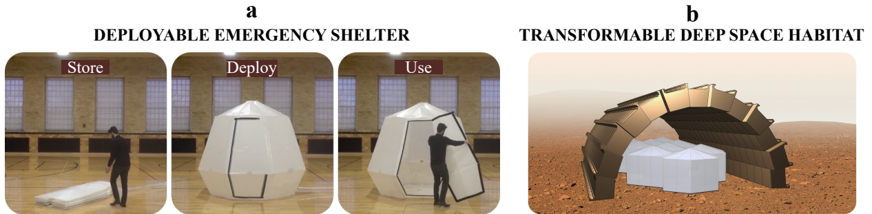
Figure 5.4: Direction 3: Applications. (a) Concept of a large-scale pressure-deployable shelter. Once inflated, because of the multistability, the pressure supply can be removed to make the internal space accessible. (b) The shelter made of stiff faces connected by flexible hinges provides physical, acoustic, and thermal barriers and could be used for emergency response in disaster zones or as a transformable habitat for deep space exploration.
