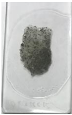
Figure 3. Thin section of an ordinary chondrite, Ochansk. A sharp irregular boundary between light and dark lithologies in transmitted light. The section size is 25 × 45 mm.
