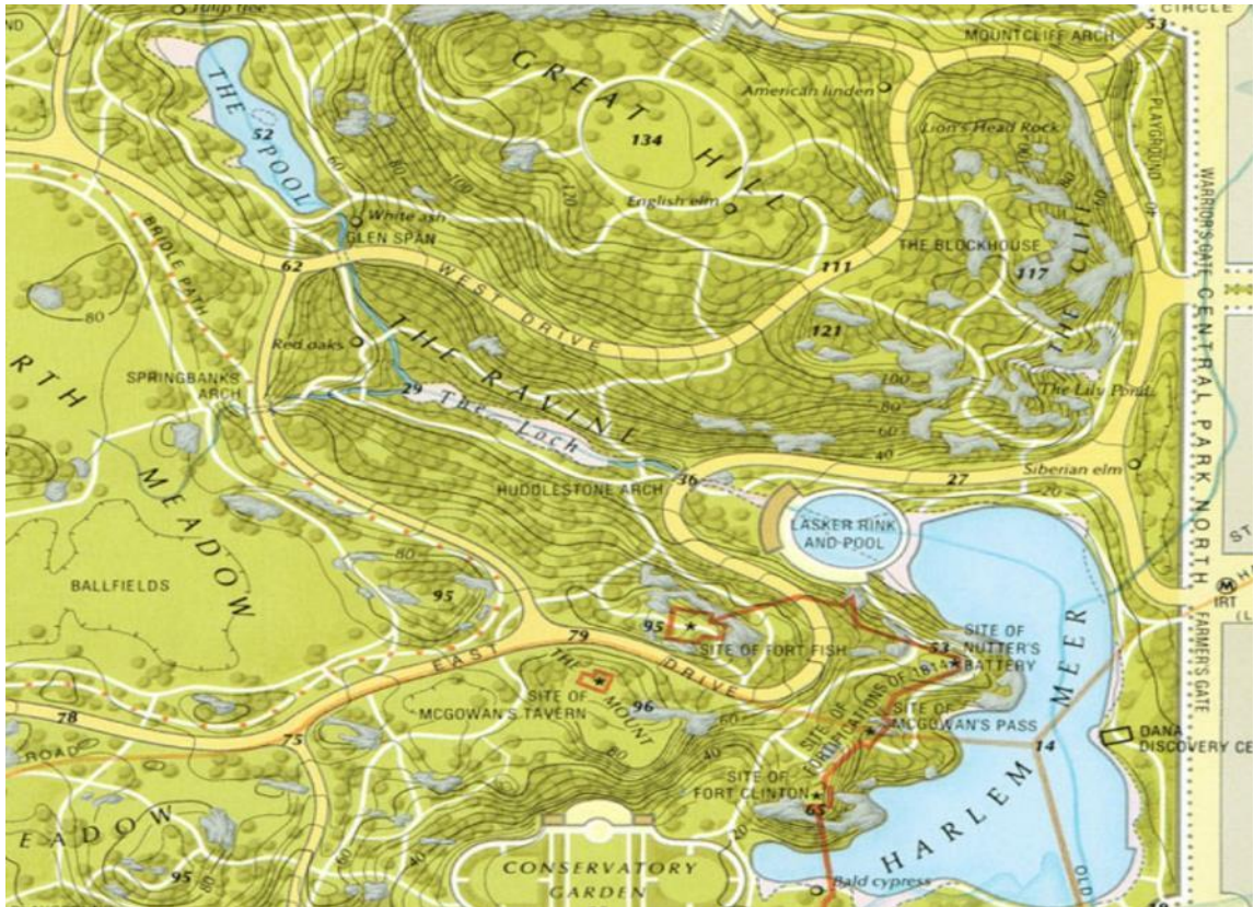
Figure 32. Topographical plan of the existing waterbodies of northern Central Park and their disrupted flow to the culvert under the Lasker Rink and Pool. The course of the historical stream: Montayne's Rivulet in 1811 is shown running through the waterbody (Greensward Foundation, 2020).
