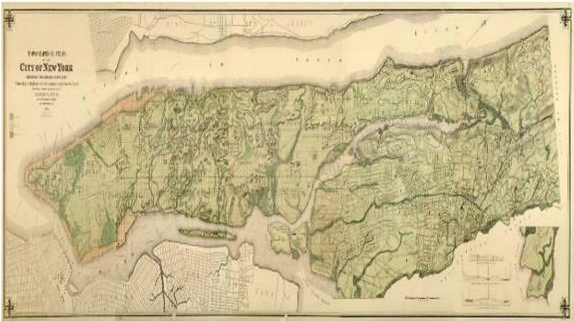
Figure 38. Topographical Atlas of the City of New York: showing original water courses and made land created by civil engineer Egbert L. Viele in 1874. (David Rumsey Cartography Associates Map Collection, 2020).
