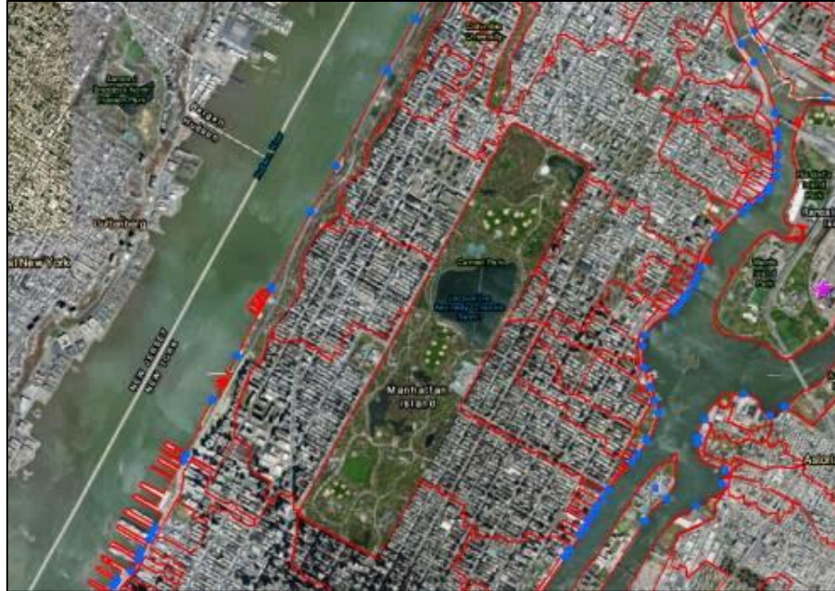
Figure 45. CSO drainage areas for Central Park and northern Manhattan (by author using ArcGIS, 2020). Data source: Open Sewer Atlas NYC and USGS.
