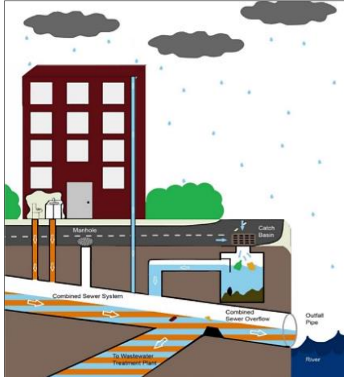
Figure 13. NYC Municipal combined sewer overflow (CSO) in wet weather (NYC EPA, 2020).
