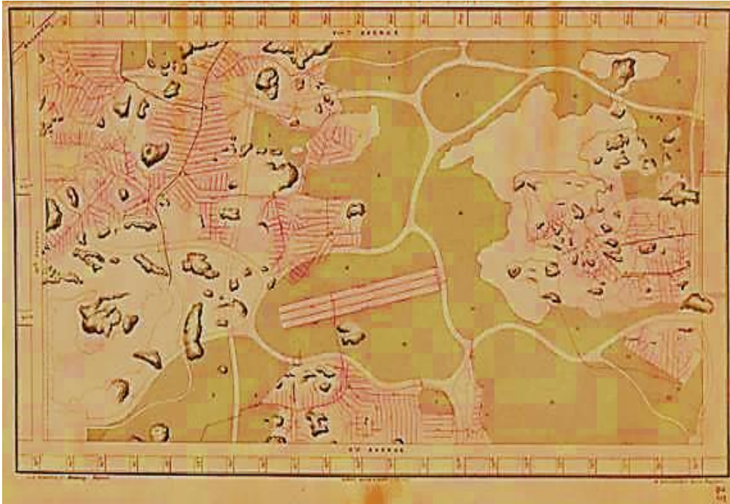
Figure 21. Drainage system on lower part of Central Park as completed up to December 31st, 1858. Compiled by George E. Waring Jr., drainage engineer (Central Park Conservancy, 2020).
