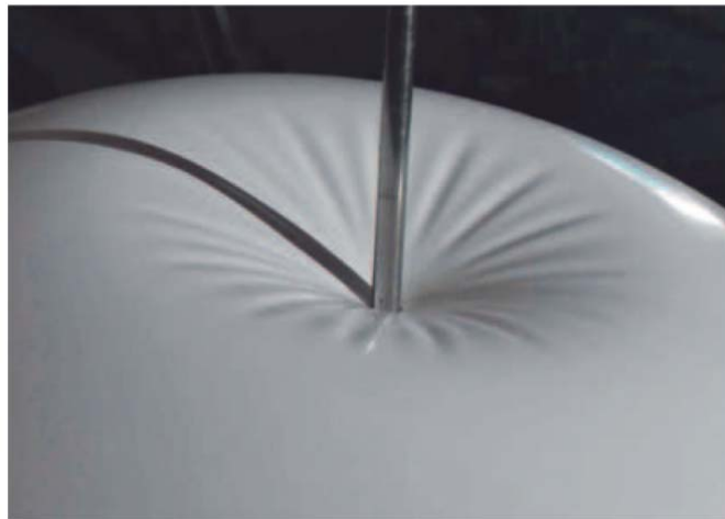
Fig. 16 Buckling of an inflated rubber ball subject to a cylindrical indenter (with permission from Vella et al [18])
