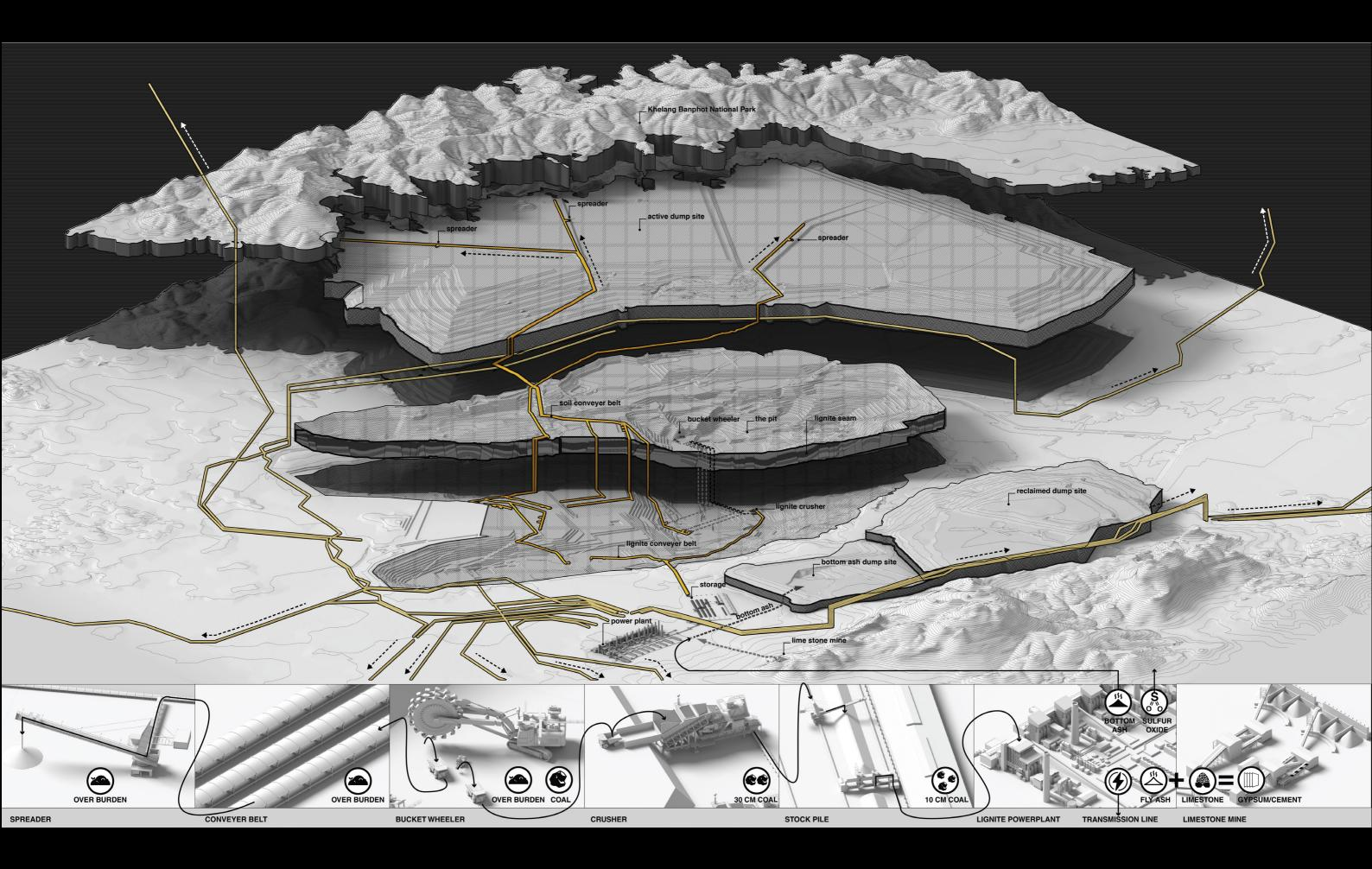
**Existing Lignite Extraction** The processing of extracting and dumping land in the lignite mining operation itself then becomes key to the design as the overburden piled up onto the dump site to form the upper reservoir.
