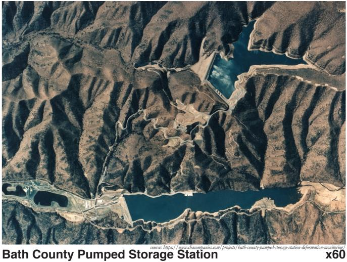
generation capacity 3,003 MW storage capacity 10 hours (24,000 MWh) 800,000 homes for 1 day
