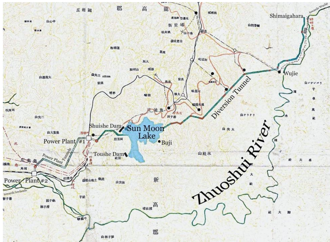
Figure 4.1: Sun Moon lake hydroelectric complex plans as of 1929; as described below, final plans differed, most significantly in moving the diversion intake from Shimaigahara to Wujie. The lines connecting the lake and tunnel sections to the north are roads, pushcar lines, electrical lines, and cable cars used for transport between construction areas and the town of Puli (埔里). Note how the multiple tunnels effectively hook Sun Moon lake into the Zhuoshui river system, diverting water away that, far downstream, eventually rejoins the river. 9
