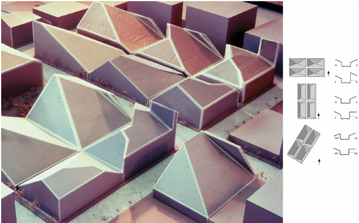
Fig.5. 9 A model of Knowles's solar envelopes in an urban context (left), the form of envelopes reflecting different street orientation (right).
