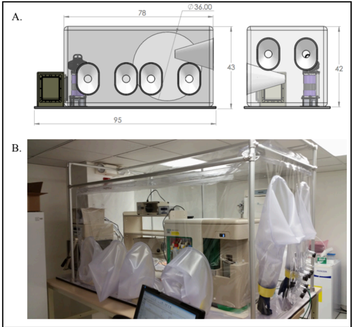
Figure 3: Custom built anaerobic FACS sorting chamber.
