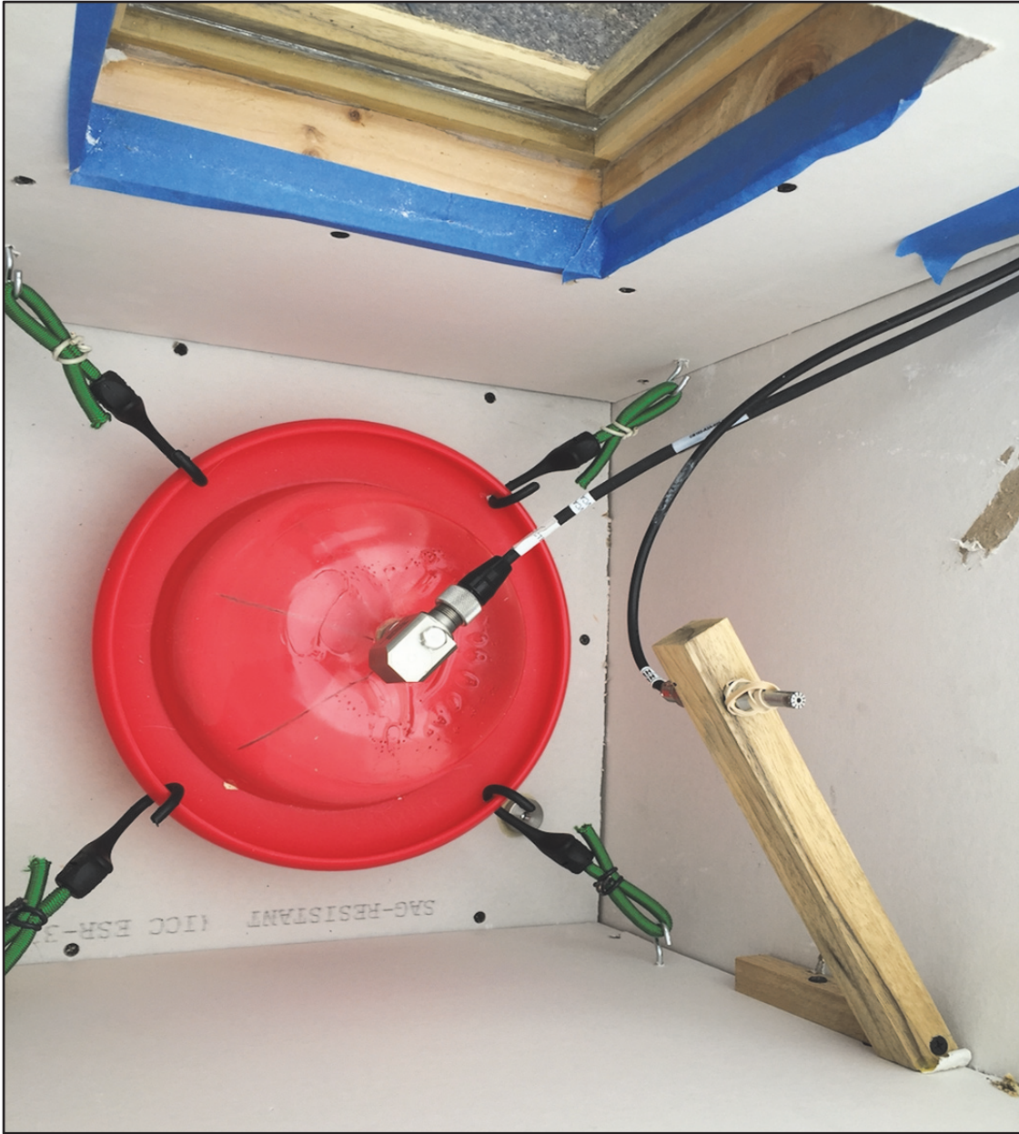
Figure 13. Instrumentation setup for the microphone and accelerometer.
