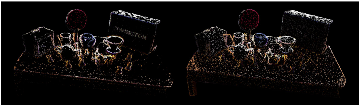
Figure 2.7: Color-aware contour-enhanced downsample (left); Color-blind contour-enhanced downsample (right). Both images contain a relatively equal number of points (approximately 8% of the original point cloud).
