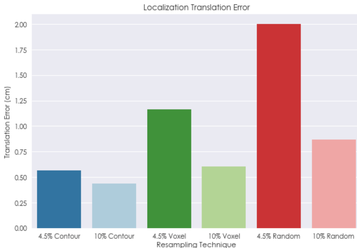
Figure 3.5: Comparison of translation error relative to ground truth for various resampling strategies. Each bar presented here is the result of averaging together 5 runs of each technique.
