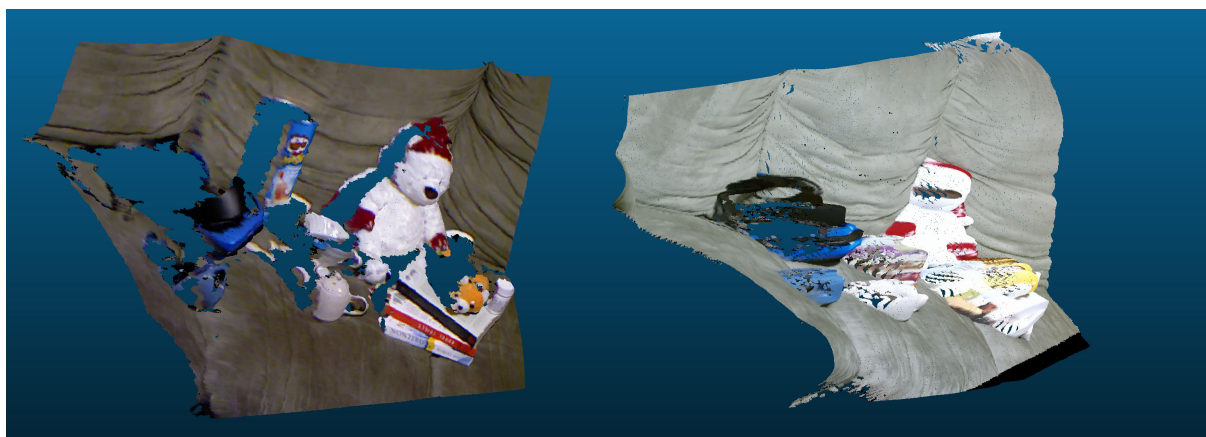
Figure 2.1: A side-view comparison of similar scenes captured by the Kinect v1 (left) and Kinect v2 (right) at depth discontinuities. The Kinect v2 demonstrates significant flying pixel effects, while the Kinect v1 accurately trims the point cloud at discontinuities.
