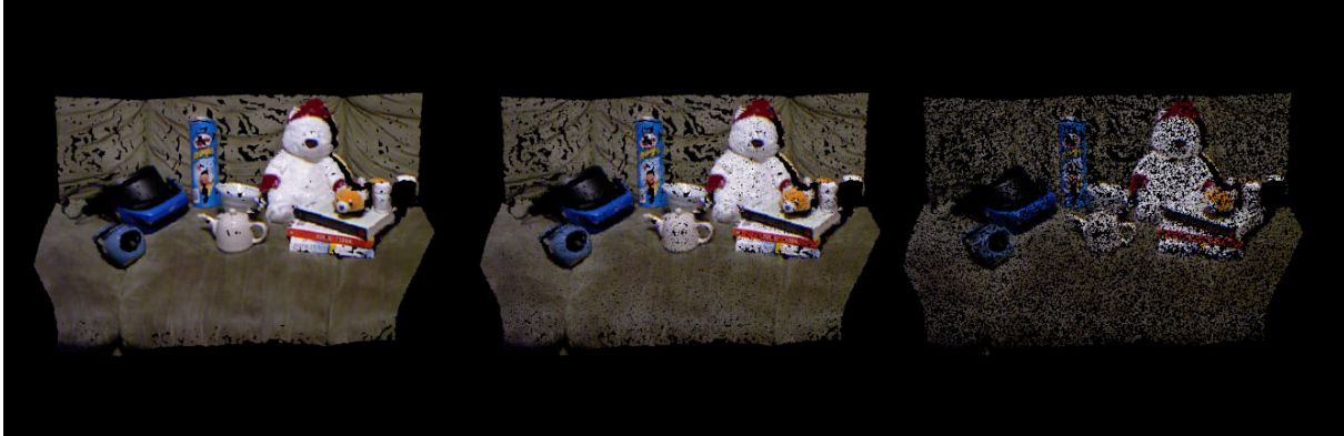
Figure 2.4: The original scan (left); Uniform random downsampling with p = 0.25 (center); Uniform random downsampling with p = 0.05 (right).
