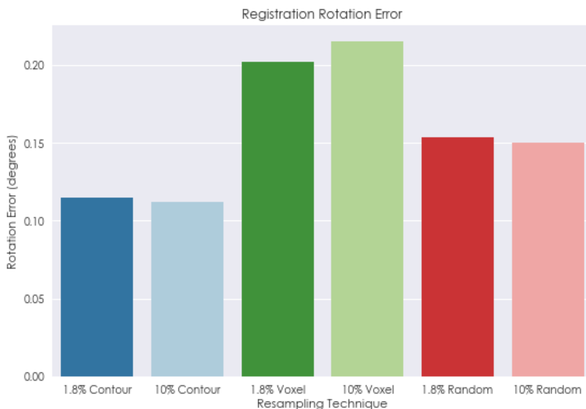
Figure 3.9: Comparison of rotational error relative to ground truth for various resampling strategies. Each bar presented here is the result of averaging together 5 runs of each technique.
