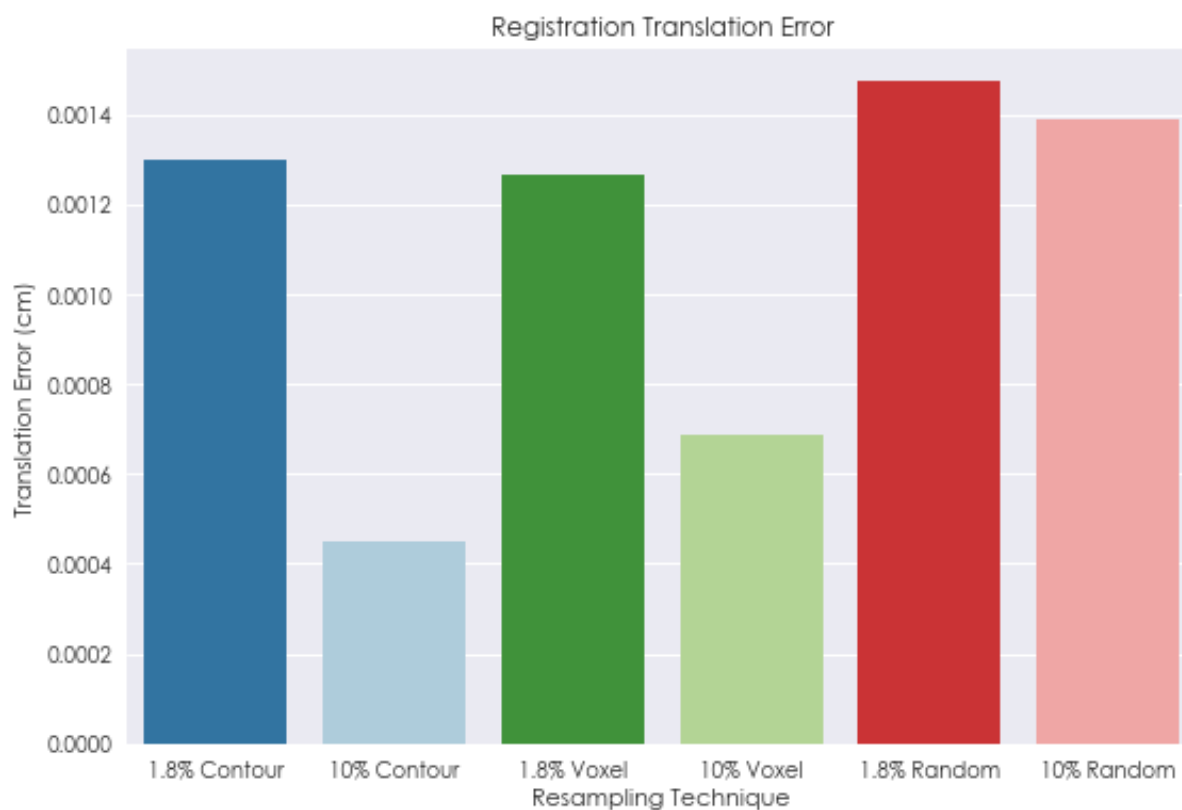
Figure 3.8: Comparison of translation error relative to ground truth for various resampling strategies. Each bar presented here is the result of averaging together 5 runs of each technique.
