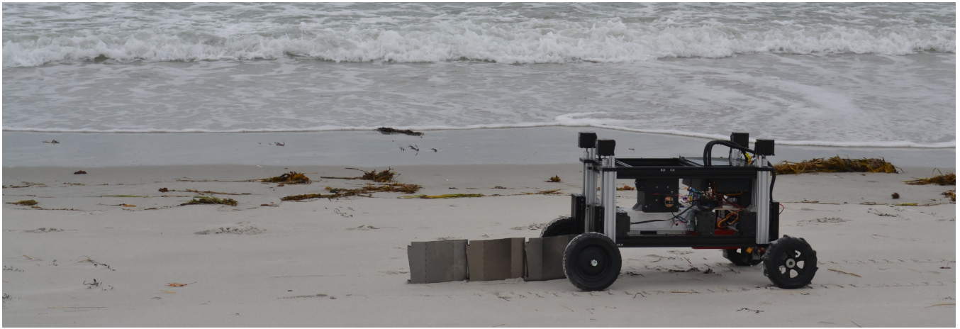
Fig. 1. Vision for Romu operating in a natural setting. Having installed the three piles it carries in one payload as the start of an erosion barrier, it heads for a supply cache to reload.
