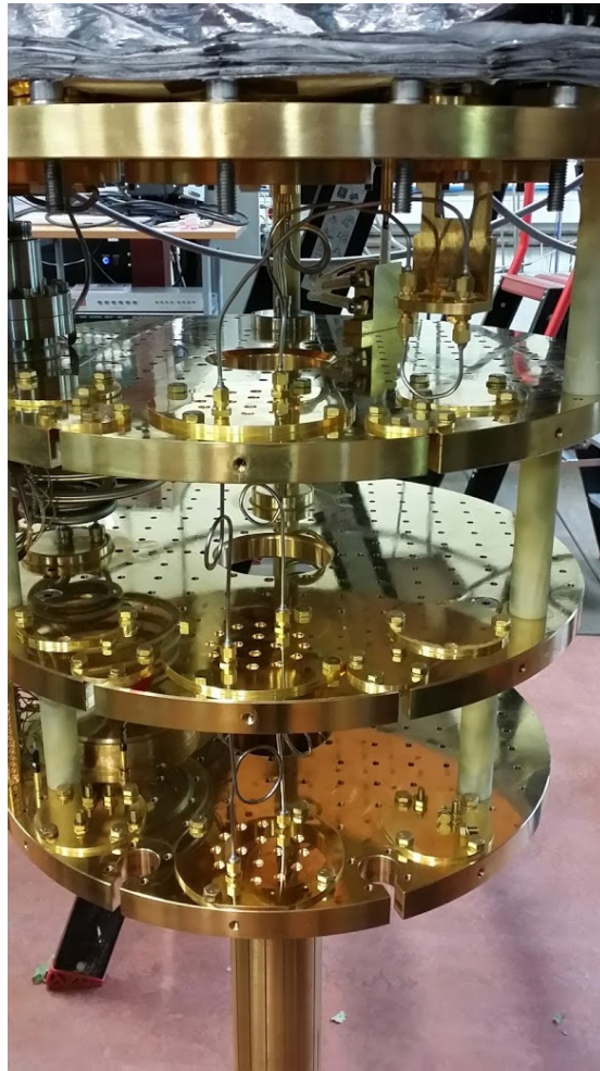
Figure A.10: Close up of the Leiden IVC plates. Starting from the top, the shown plates are the 4\text{ K} , still, 100\text{ mK} , and mixing chamber plates. The still is the silver piece seen on the left side of the image mounted on the top side of the still plate. Image taken in Leiden, Netherlands while constructing the fridge. At the bottom of the image, the “tail” that extends down into the magnet bore can be seen
