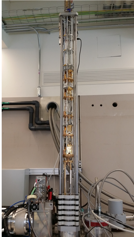
Figure A.12: Image of the insertable, top-loading probe built for the Leiden dilution refrigerator with the retractable bellows lowered. Each gold plated copper section mechanically expands once inserted to thermalize to a stage in the main fridge body. Near the bottom of the probe, and extender is seen which, during operation, contains the sample and is lowered into the magnet bore.
