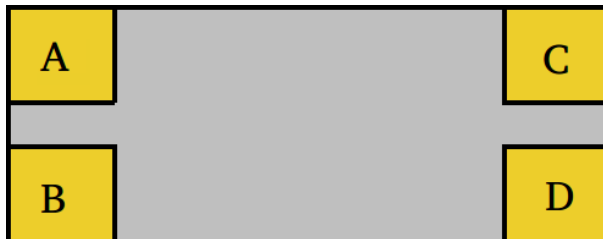
Figure 2.28: Cartoon of a four-terminal device. If the voltage between terminals A and C is cross-correlated to the voltage between terminals B and D, the result will be more sensitive to the temperature of the device than pairing A-B and C-D
