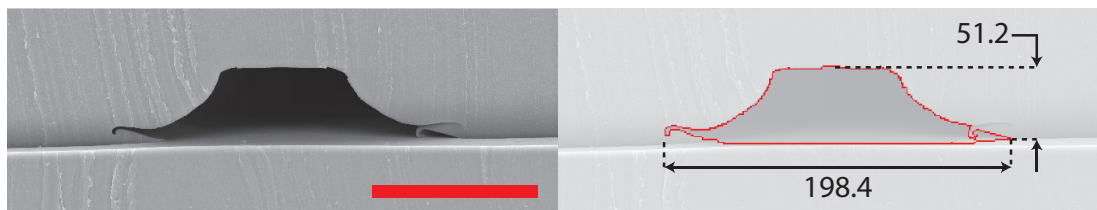
Figure 4.11: SEM image of 50 \times 50 \mu\text{m} channel exposed at 150 \text{ mJ}/\text{cm}^2 . Notice the sharp corners at the top of the channel. (Left) Original SEM image. (Right) SEM image with channel highlighted and dimensions added. All dimensions are in micrometers. Scale bar is 100 \mu\text{m} .
