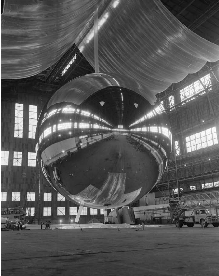
Figure 4.26. ECHO 1 satellite, test inflation in dirigible hangar before launch on August 12, 1960. Photo: NASA.
